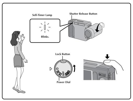
Turn the Power Dial, while pressing its Lock Button, to " $\circ$ ".
